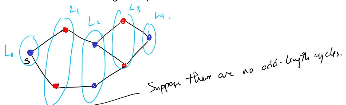
Proof by algorithm. Pick some starting vertex  $s$  and run a BFS from  $s$ , generating layers  $L_0, L_1, L_2, \dots$
